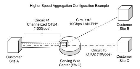
In the example of a higher speed aggregation arrangement depicted in the diagram above, there are three AT&T Dedicated Ethernet circuits, as follows:
