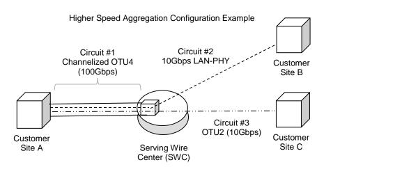
In the example of a higher speed aggregation arrangement depicted in the diagram above, there are three AT&T Dedicated Ethernet circuits, as follows:
