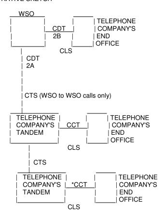
CTS: Carrier tandem Switching CLS: Carrier Line Switching CDT: Carrier Dedicated Trunk CCT: Carrier Common Trunk WSO: Wireless Switching Office
