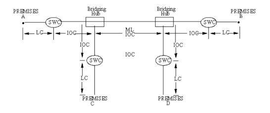
LC = Local Channel IC = Interoffice Channel<sup>(1)</sup> B = Bridging<sup>(1)</sup> SWC = Serving Wire Center ML = Mid-Link
