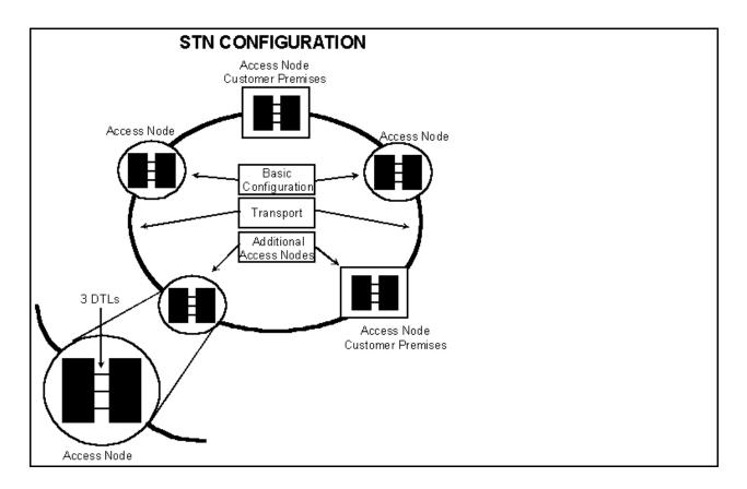
This configuration depicts an STN arrangement using the Basic Configuration equipped with DTL Volume Option 3 which includes three Access Nodes and three DTLS, plus two Additional Access Nodes.
