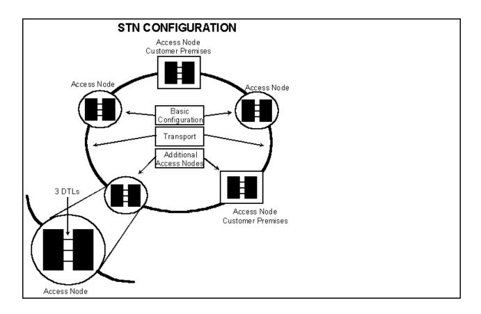
This configuration depicts an STN arrangement using the Basic Configuration equipped with DTL Volume Option 3 which includes three Access Nodes and three DTLS, plus two Additional Access Nodes.
