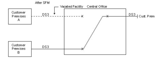
Note 1: This facility may exist as a result of an order for MegaLink Custom (DS3) service concurrent with the SFM request or, in the case of virtual collocation, as a cross-connect arrangement requested by the interconnector.
