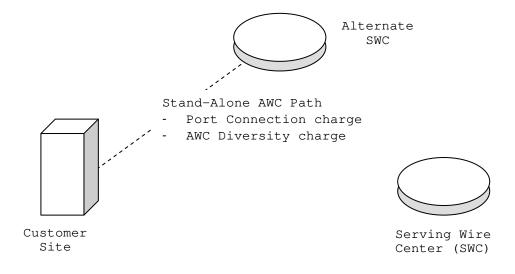
The Port Connection is routed to a SWC other than its normal SWC in a Stand-Alone AWC arrangement.
