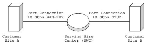
This example illustrates a same speed / different format circuit configuration where there is a 10Gbps WAN-PHY Port Connection between Customer Site A and the serving wire center and a 10Gbps OTU2 Port Connection between Customer Site B and the serving wire center. In this circuit example, both a 10Gbps WAN-PHY and a 10Gbps OTU2 Port Connection charge would apply.
