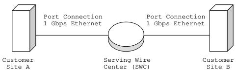
This example illustrates a 1 Gbps Ethernet circuit from Customer Site A to Customer Site B for a same speed / same format arrangement. In this example, two - 1 Gbps Ethernet Port Connection charges are applicable.
