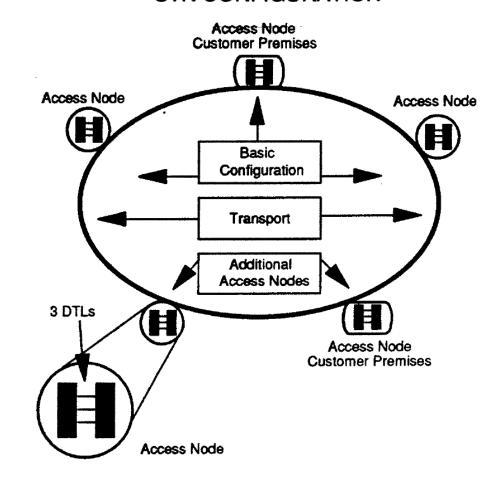
This configuration depicts an STN arrangement using the Basic Configuration equipped with DTL Volume Option 3 which includes three Access Nodes and three DTLs, plus two Additional Access Nodes.
