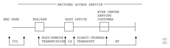
CCL: CARRIER COMMON LINE LS: LOCAL SWITCHING EF: ENTRANCE FACILITIES RS5/RSM: REMOTE SWITCHING SYSTEM/REMOTE SWITCHING MODULE
