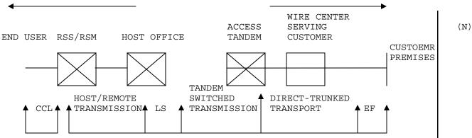
CCL:CARRIER COMMON LINE LS:LOCAL SWITCHING EF:ENTRANCE FACILITIES RSS/RSM: REMOTE SWITCHING SYSTEM/REMOTE SWITCHING MODULE
