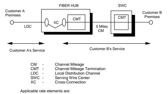
Local Distribution Channel - Customer A Local Distribution Channel - Customer B Cross-Connection - DS3 to DS3 5 Miles Channel Mileage - Customer B 2 Channel Mileage Terminations - Customer B
