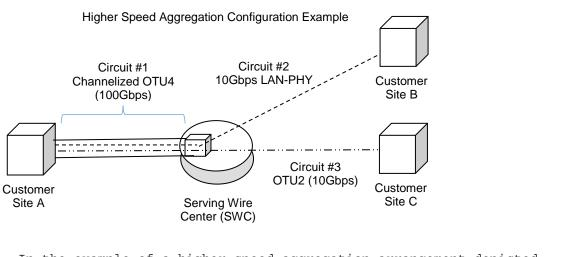
In the example of a higher speed aggregation arrangement depicted in the diagram above, there are three AT&T Dedicated Ethernet circuits, as follows:
