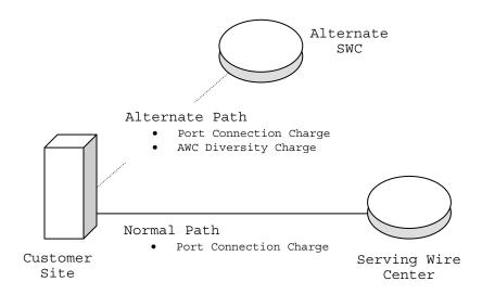
(ii) Stand-Alone Alternate Wire Center (AWC) Routing Alternate Wire Center Diversity is available as a standalone AWC arrangement where there is no actual diversity. In this arrangement, an AT&T Dedicated Ethernet Port Connection is routed to an alternate wire center rather than its normal serving wire center.
