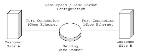
This example illustrates a 1Gbps Ethernet circuit from Customer Site A to Customer Site B for a same speed / same format arrangement. In this example, two - 1Gbps Ethernet Port Connection charges would apply.
