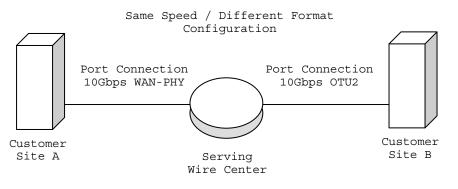
This example illustrates a same speed / different format circuit configuration whereby there is a 10Gbps WAN-PHY Port Connection between Customer Site A and the serving wire center and a 10Gbps OTU2 Port Connection between Customer Site B and the serving wire center. In this example, both a 10Gbps WAN-PHY and a 10Gbps OTU2 Port Connection charge would apply.
