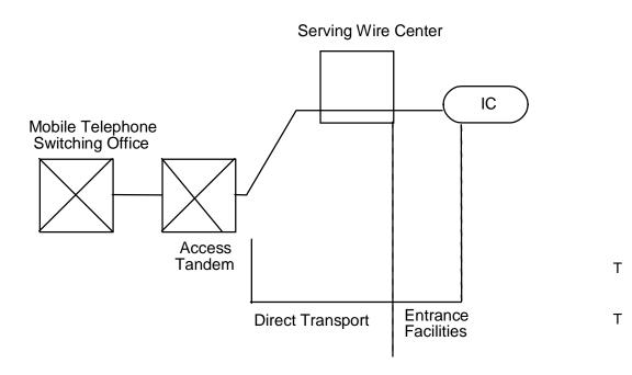
Cellular Mobile Carrier Interconnects with Local Exchange Carrier at the Access Tandem
